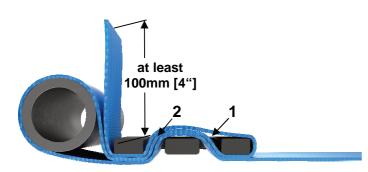
4. Check again for proper shoulder belt tilt lock adjuster positioning and for the 3-bar slide to be as close as possible to the roll cage bar or end bracket.
