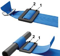
3. Make sure the strap end protrudes at least 100 mm [4"] or even longer from slot 2. If it is less than 100 mm [4"] disassemble and start over again. If longer, roll in the strap end and fix it by a cable tie to the shoulder belt.
