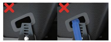
Risk of severe injuries or death. Sharp edges may cut the webbing and the racing harness may fail during an accident. Never run straps over sharp edges and brackets.
