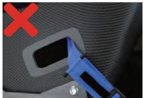
This webbing runs too far back, and at too low of an angle. A Lap belt cannot be routed straight through seat slots. It will tend to slide off the pelvic bone and result in submarining. This will also add additional load to the anti-sub strap. Severe injuries or death may occur.
