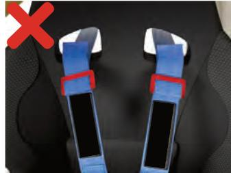
Risk of severe injuries or death. 3-bar slides positioned in such a way may cut into the occupant's neck during an accident. Never install a racing harness with attachment hardware [such as the 3-bar slide pictured at left] next to the occupant's body or to tor on the inside of the seat openings.
